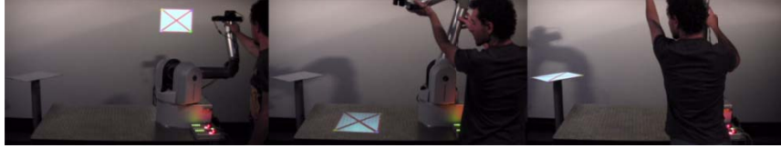
Fig. 5. Active Projection. The snapshots show how the user physically interacts with the robot for finding a suitable projection plane. The system aims to project a fixed size undistorted image following the geometric perspective of the projected surface
