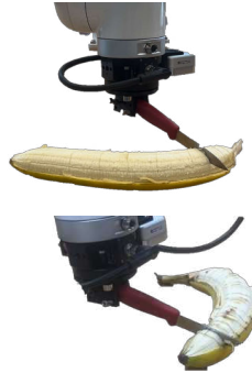
Figure 3: Shape-invariant task representation and transfer using DOF. (A) (i) An object-centric trajectory (gray) composed of an approaching phase and a surface-following phase. Small reference frames are the object-centric local reference frames represented by DOF, while the large dashed frame denotes a single body-fixed frame. (ii) Gray trajectory is expressed in object-centric local frames (solid lines) and the single body frame (dashed lines). (B) Local action primitives providing shape-invariant task descriptions in object-centric local reference frames. (C) Simulated visualizations showing the keypoints (blue), tool paths (black), and the x-axis of local frames (red). (D) Real-world experiments showing transfer of slicing, peeling, and tactile coverage tasks to novel objects.
