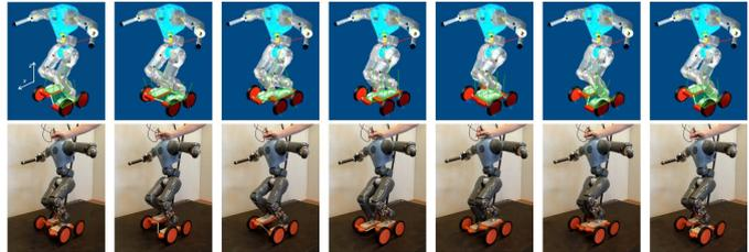
Figure 14: One period of COMAN steady-state pedaling on a pedal racer in *Webots* dynamic simulator (top) and in experiment (bottom).
