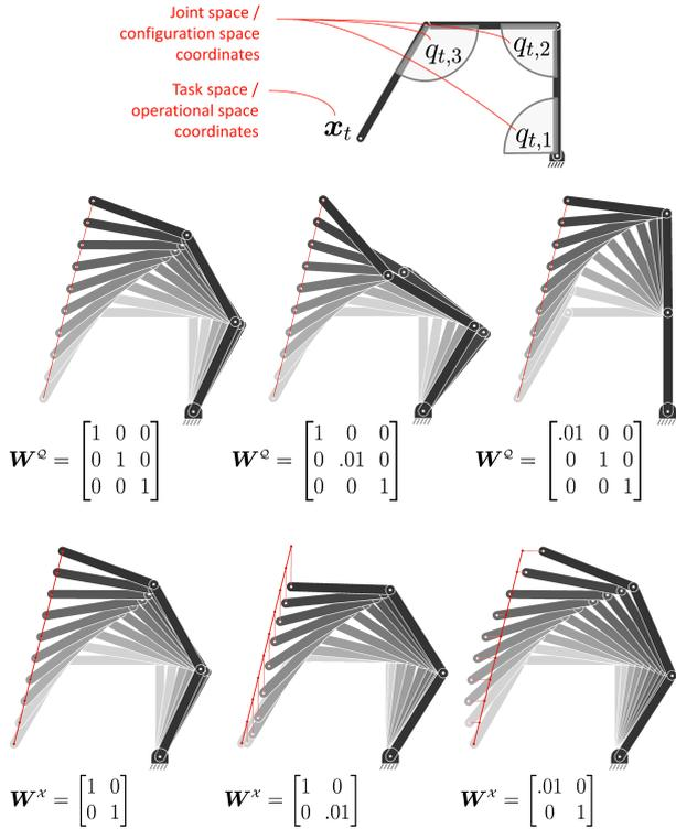
Figure 16: Task prioritization based on a weighted least squares estimate of inverse kinematics. *Top*: Variables involved. *Middle*: with weights in joint space (with right pseudoinverse  $\hat{q}_t = W^o J^T (J W^o J^T)^{-1} \dot{x}_t$ ; see also (5)). *Bottom*: with weights in task space (with left pseudoinverse  $\hat{q}_t = (J^T W^x J)^{-1} J^T W^x \dot{x}_t$ ; see also (4)).
