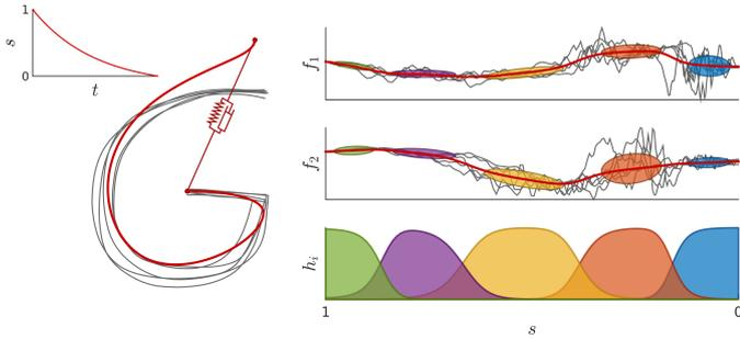
Figure 3: DMP with a GMM to encode the joint distribution of forcing terms  $\mathbf{f}(s)$  and phase variable  $s$ .
