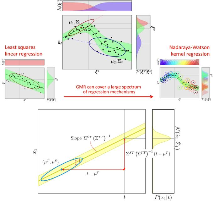
Figure 6: Gaussian mixture regression (GMR) has a simple formulation that can cover a wide range of regression techniques, from multiple multivariate linear regression (single Gaussian) to data-driven kernel-based regression (Gaussian centered on each datapoint).
