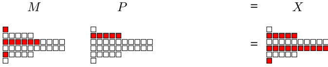
(a) Using the geometric product results in both blades of lower and higher grade.
