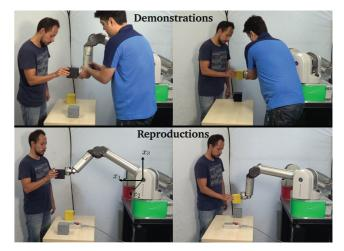
Fig. 2: Experimental setting of the human-robot transportation task: (*top*) kinesthetic demonstrations, and (*bottom*) reproduction phase.
